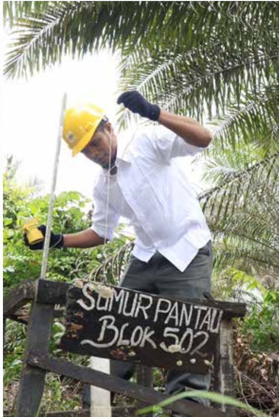
Monitoring groundwater levels in peatland areas at Tanjung Makmur Estate, West Kutai, East Kalimantan
