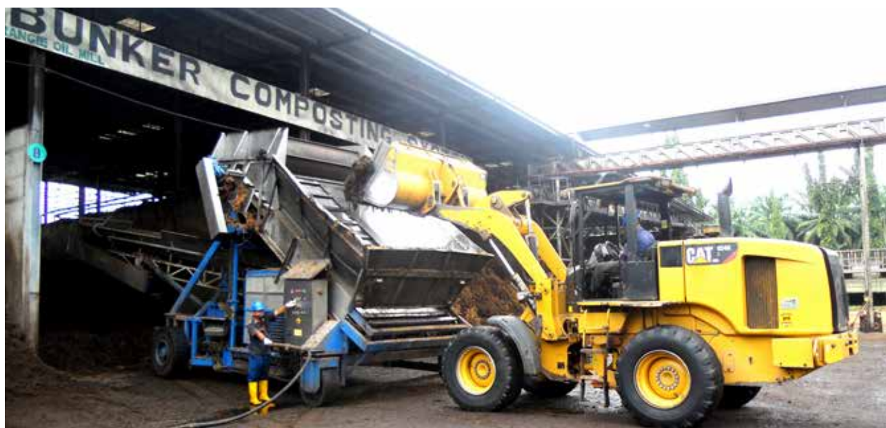
Aerated Bunker Composter in our Turangie Mill, North Sumatra Aerated Bunker Composter di Pabrik Kelapa Sawit Turangie, Sumatera Utara
